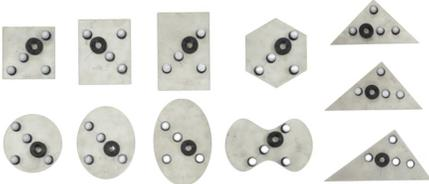
Figure 3: **Out-of-distribution objects.** These objects, made of a different material, stainless steel, are much heavier and have different shapes compared to the 250 objects used to build our meta-learning dataset. Their mass distribution is uniform. More details on these objects can be found at Yu et al. (2016).
