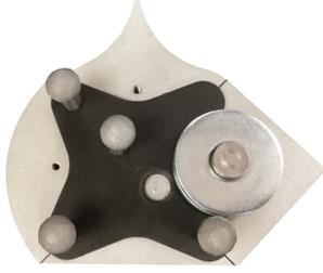
Figure 2: **Object made of the four possible sides.** Weights can be attached in the holes. There is an extra hole in the triangle, covered by the wafers. From right to bottom, the sides of the shape are triangle (94.1g), concave (74.1g), circle (67.5g) and rectangle (31.2g). Following our convention for naming objects, we denote this object as '2C1a3a4a'.
