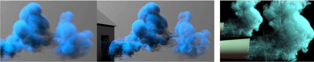
Figure 1: Two examples of high resolution flows generated by our network: on the left, a flow around an obstacle, with the coarse input on the left, and the high resolution output on the right. The output in this case has almost 200 million degrees of freedom. On the right a jet flow example with an output resolution of  $512^3$  is shown. In this case, the low-resolution input is shown in the top-left inset image.
